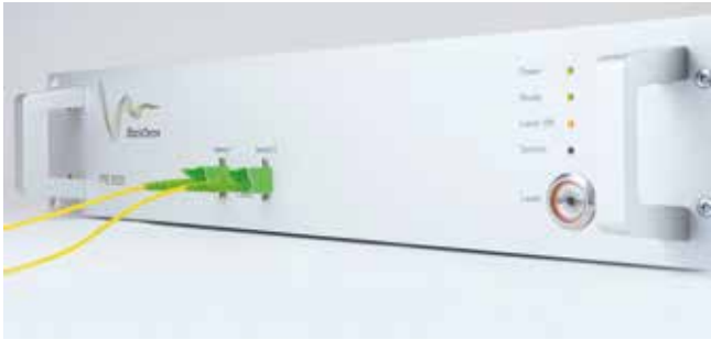
Figure 8: A fibrisTerre distributed fiber optic sensing interrogator unit
