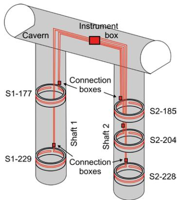
Figure 8: Distributed fiber optic measurement system at Götritz access (not to scale)
