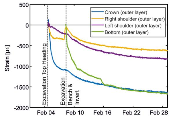
b. Strain evolution in the outer shotcrete layer
