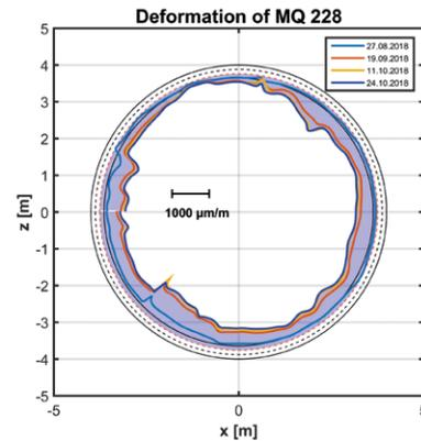
Figure 9: Strain distribution in the inner layer of the shotcrete lining (section S2-228) at different dates from the zero measurement on 21.08.2018
