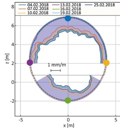
a. Strain distribution in the outer shotcrete layer along a tunnel cross section
