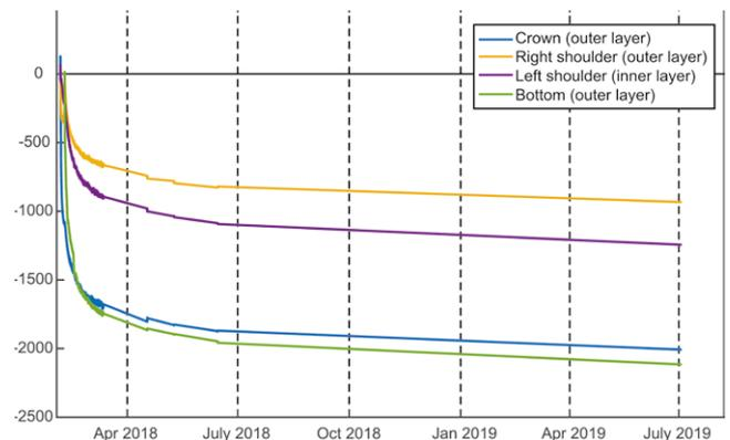
Figure 6: Long-term strain development of tunnel lining
